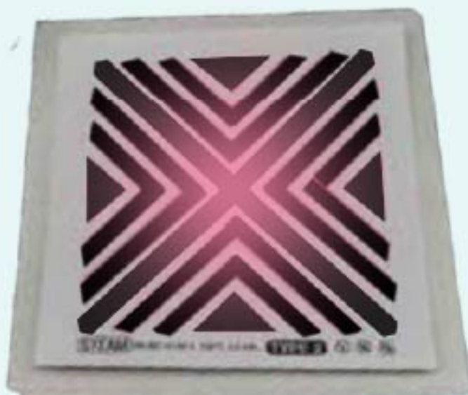
FAIL: insufficient air removal
